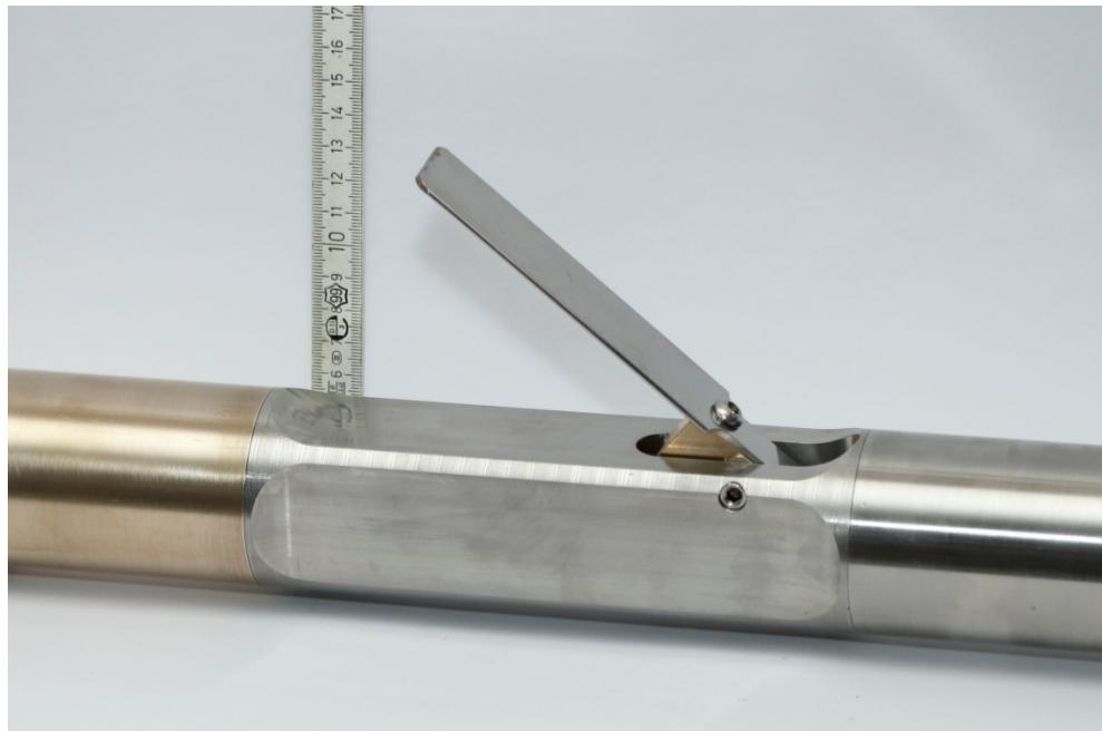
**Fig. 5 Sonde with standard steel clamping arm**
