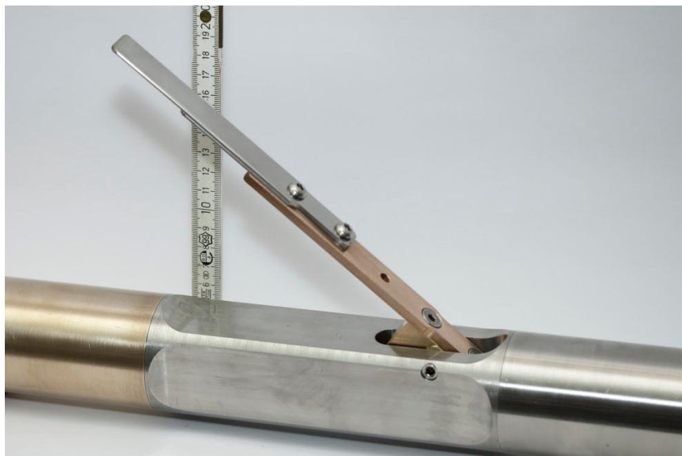
**Fig. 7 Extended clamping arm for 200 mm boreholes**
