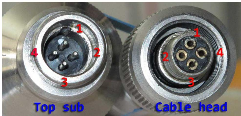
Fig. 8 Gearhard Owen 4-pin cable head connectors
